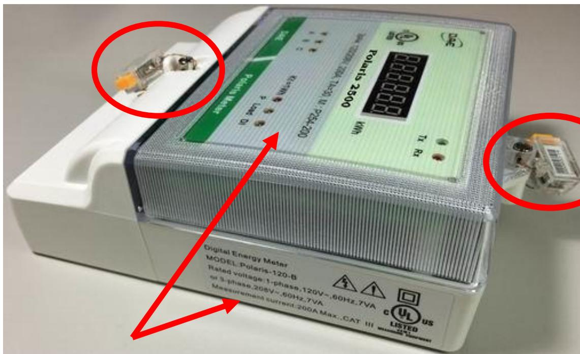
Side View of Meter with Front and Side Identification and Sealing Provisions
