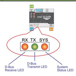
Note: The system status will flash once a second during normal operation. The other LEDs will only flash when there is activity
